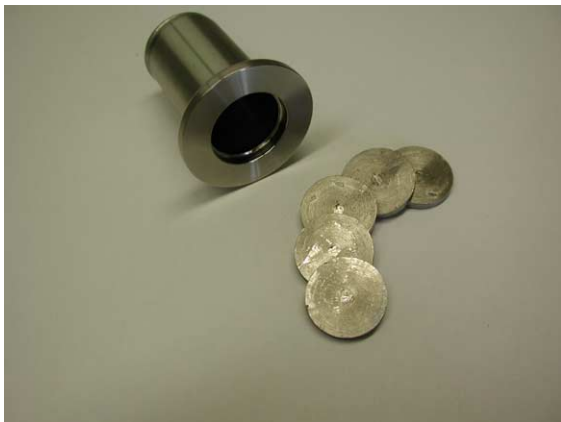
Fig. 1. Austenitic steel container with a bottom of T91 steel constructed for irradiation of 16 mm \varnothing LBE discs.
