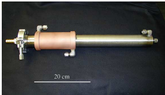
Fig. 2. Apparatus for investigating the evaporating behaviour of irradiated LBE.
